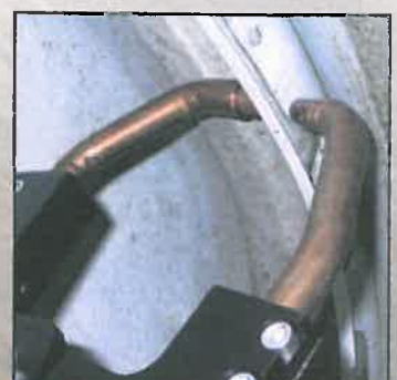
X-Adapter Arm is a must for tight areas with limited space for the electrodes.
